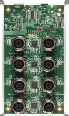
Figure 3. MAXREFDES145# 8-Port IO-link master reference design
