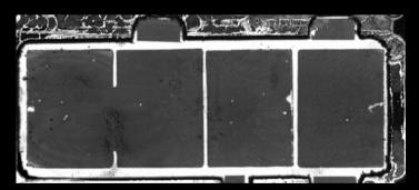
Figure 3 Ultrasound analysis of solder connection between DBC and baseplate
