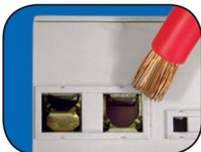
Cage-clamp terminals from 45 to 90A guaranteeing secure connection of cables up to 25mm 2 — AWG 3 (Midi & Power only)
