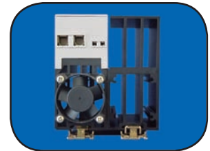
Mounting holes for forced air cooling (Midi & Power only)
