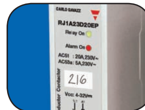
Identification window and LED indication of input status and optional over-temperature alarm status
